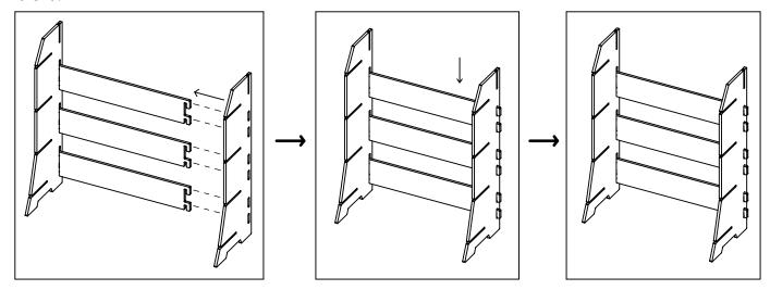
**STEP 3:** Insert the Bottom Shelf into the bottom slots on the Side Panels. *Note: If needed, using a rubber mallet (sold separately), gently tap the parts into place.*
